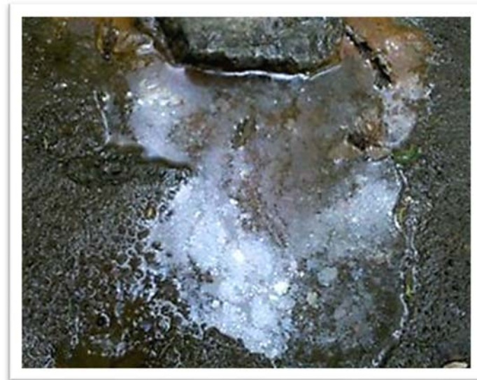
A petroleum sheen will swirl and reform itself rather than break apart.
